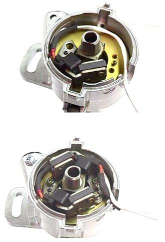
Now that the plate is located, one of the rubber bushing previously cut off the old module wires must be fitted to the new wires.
