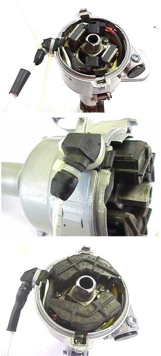
adjusted and you are done. A smaller gap will result in a spark at a lower RPM than with a larger gap. The factory gap setting is 0.008" - 0.016". Be sure that any play in the shaft is taken into account when setting the gap. The side play should not put the gap out of the tolerance range.
