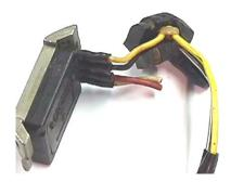
Now it is time to test fit the wired Pickups into the distributor. The first pickup is located approximately as shown with the wire looping around as shown. Use the 8-32 screws supplied with the kit. They will be tight the first time used, as the tolerance on the threaded holes is aircraft standards not automotive. Do not over torque, as the plate is aluminum. The screws are longer and thread the entire thickness of the plate
