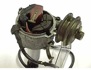
you will be able to set one of the pickup locations to the same place. This mark is only close to the final position, as the removal of the Vacuum advance will result in slight repositioning for the best position. This is covered later in the instructions.
