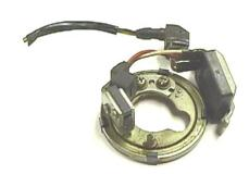
Grind, or cut and file the end of the pickups off as shown here. Make both pickups like the one on the right. If grinding, do not allow excessive vibration to damage the unit. Be sure to remove all the metal particles from the magnet areas.
