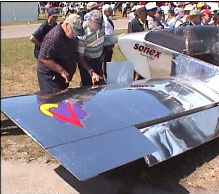
5. After working one area, move on to the next area, and so on. When through with buffing for the day, thoroughly clean the surface of any F9 polish residue around fasteners/seams/ joints, etc. Long nap microfiber cloth is very effective when polish is still fresh, and seems to have an affinity for the accumulated polish. Leaving the polish to dry makes the residue harder to remove, and may require mineral spirits.
